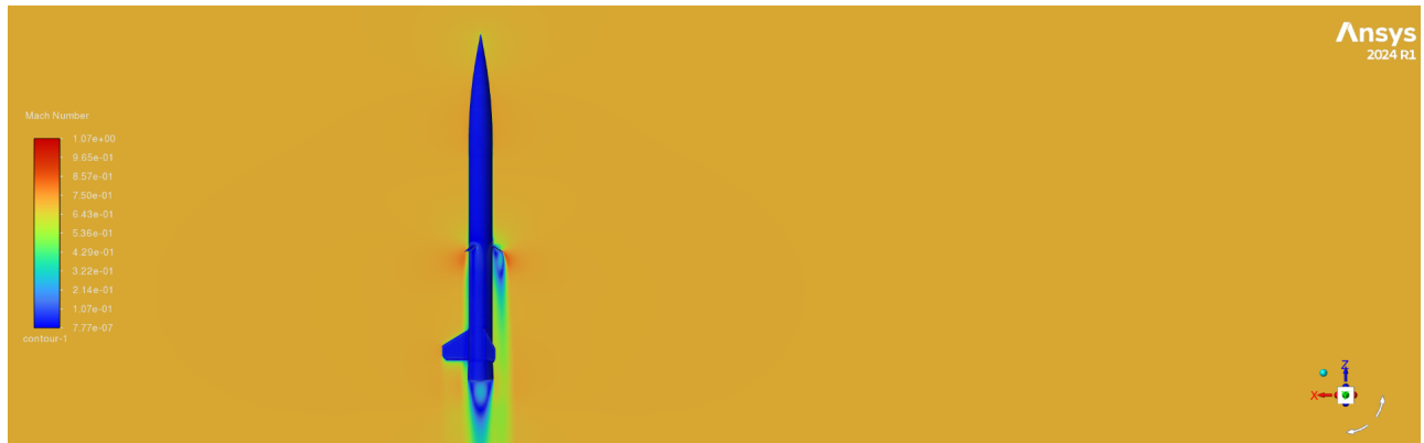
Fig. 6 Mach number contours at 80° deployment and Mach 0.7, showing local acceleration near flap edges.
