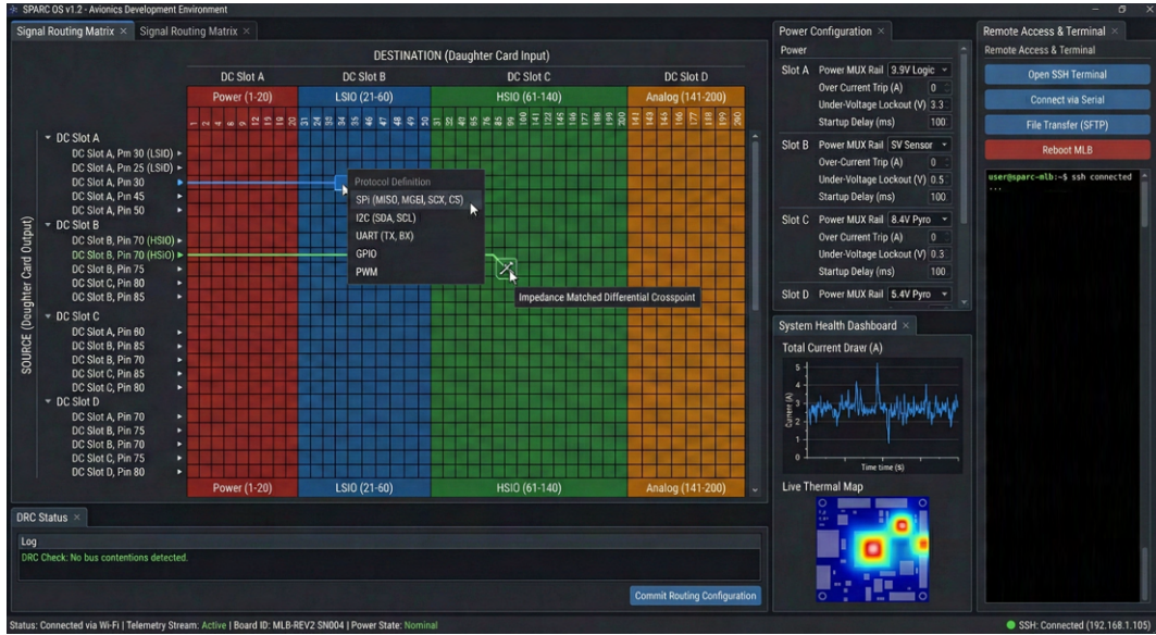
Fig. 11 SPARCOS Custom User Interface showing the signal routing matrix, power configuration parameters, and real-time system telemetry.
