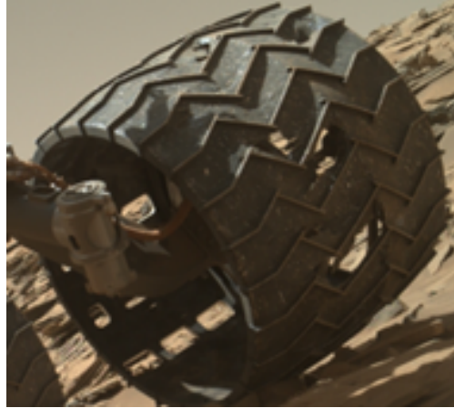
Fig. 2 MAHLI full-wheel imagery of Curiosity's left-middle wheel taken on April 18, 2016, from Ref. 12.
