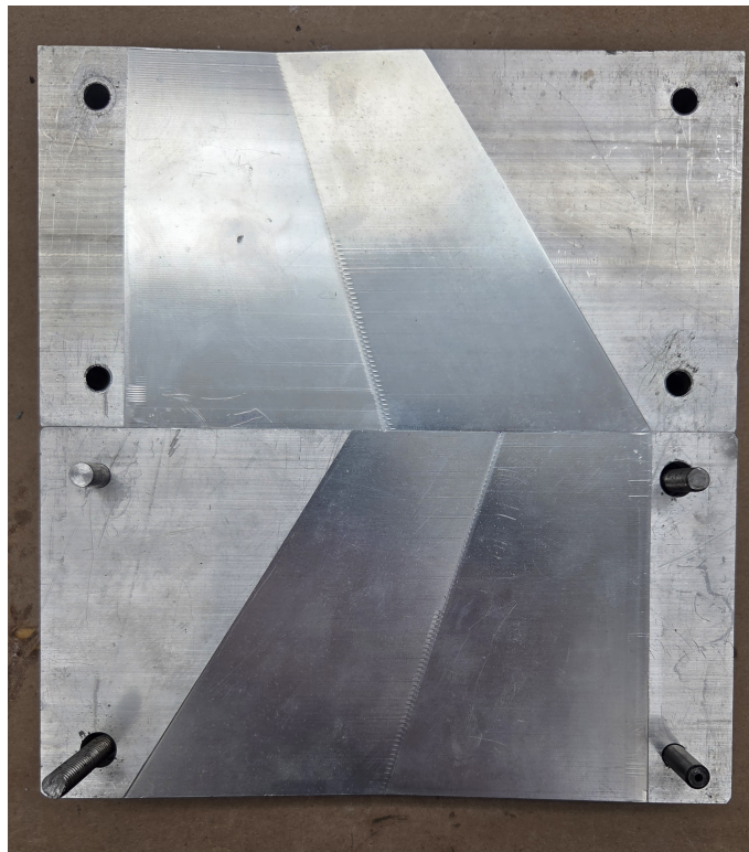
(c) CNC-machined aluminum mold assembly
