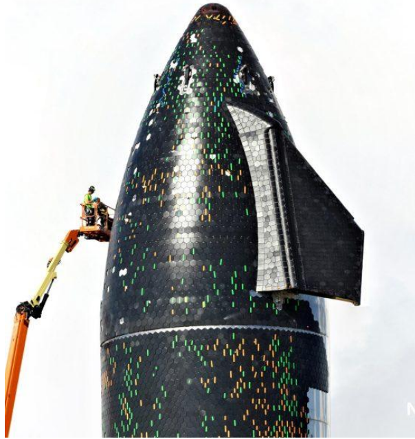
Fig 3: Close-up view of SpaceX's Starship windward surface. This shows how during ground processing, the hexagonal ceramic thermal protection system (TPS) tiles installed across the vehicle. [11]
