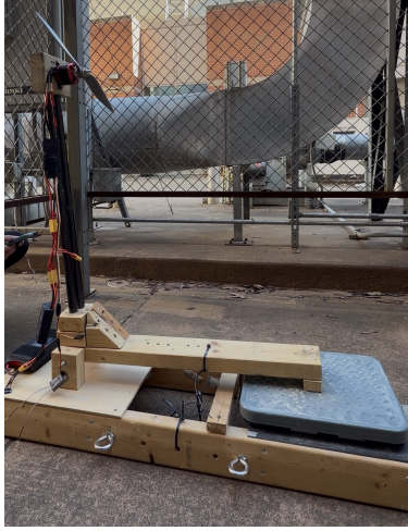
(a) Front motor and propeller mounted on thrust stand
