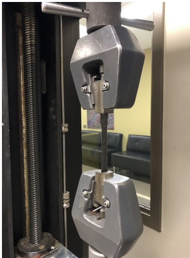
(a) Test specimen in load frame
