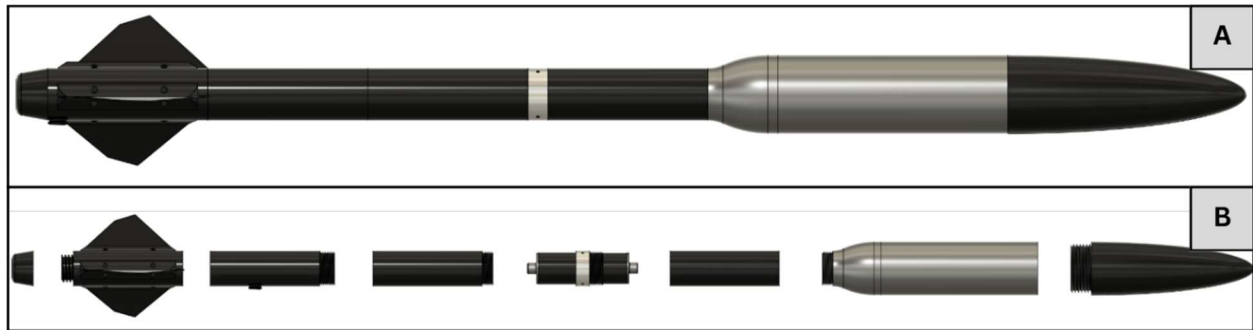
Fig. 1 Modeled Launch Vehicle (A) and Exploded View of Structural Segmentation (B)
