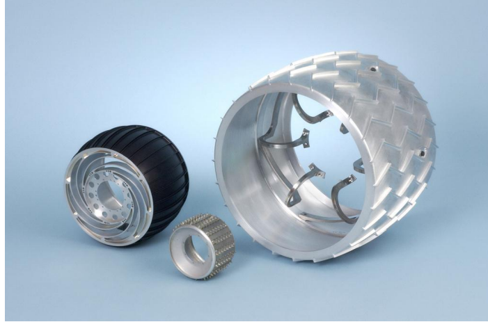
Fig. 2 Isometric comparison of Mars rover wheel sizes. Sojourner (center), Spirit/Opportunity (left), and Curiosity (right), illustrating the progression toward larger wheels across missions. (NASA/JPL-Caltech, public domain)
