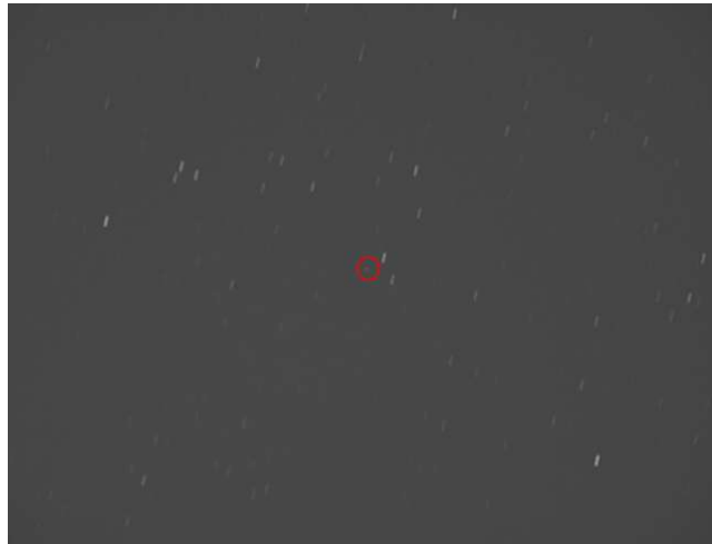
Figure 2. Unresolved image taken in orbit following mode with stationary RSO captured circled.
