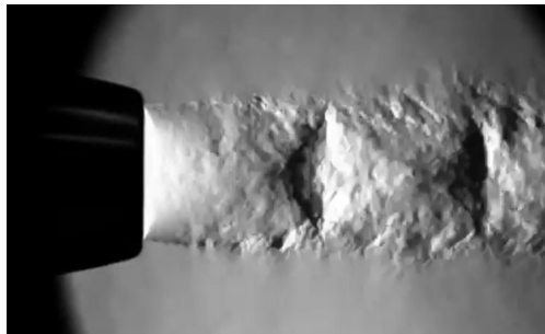
Fig. 14 Schlieren imaging of the converging-only nozzle at an upstream pressure of 70 psig.
