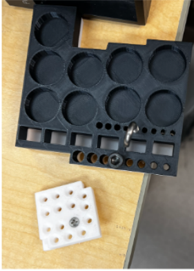
Fig. 15 Test pieces used to size 3D printed bores
