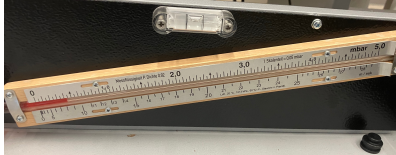
(b) Velocity measurement and manometer panel.
