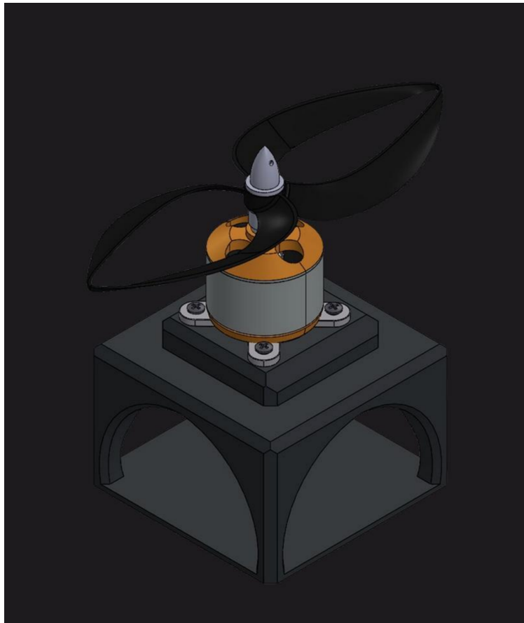
Fig. 2 Custom static thrust stand featuring a topology-optimized motor mount (FoS=2.5).
