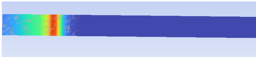
Fig. 6. Pressure-gradient field from the initial ANSYS CFX simulation showing two interacting compressive structures during early propagation. The right-running detonation front is displayed and a secondary left-running compressive wave generated by boundary interaction is displayed in Fig.10. t = 0.69985 \text{ ms} .
