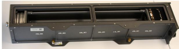
**Fig. 18 Nanoracks Deployer with Panels Removed**
