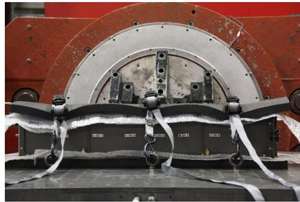
**Fig. 15 RHOK-SAT in the deployer while mounted on a vibration apparatus, simulating conditions satellite will experience in Cygnus while en route to the ISS.**
