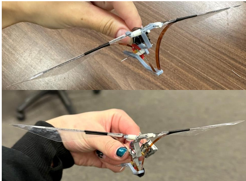
Fig. 8 Design A resin (Top) and PLA (Bottom) assembled vehicles.
