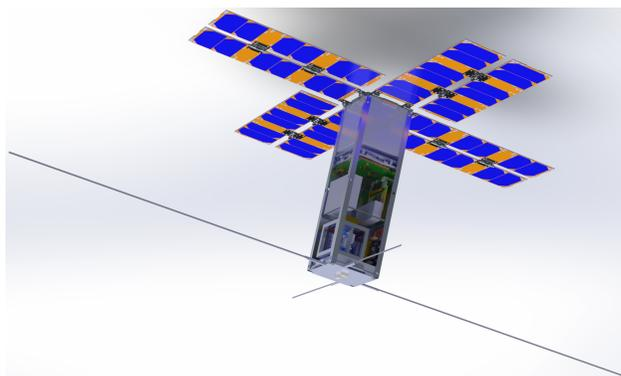
Figure 7. CLEOSATRA isometric view (side panels removed)
