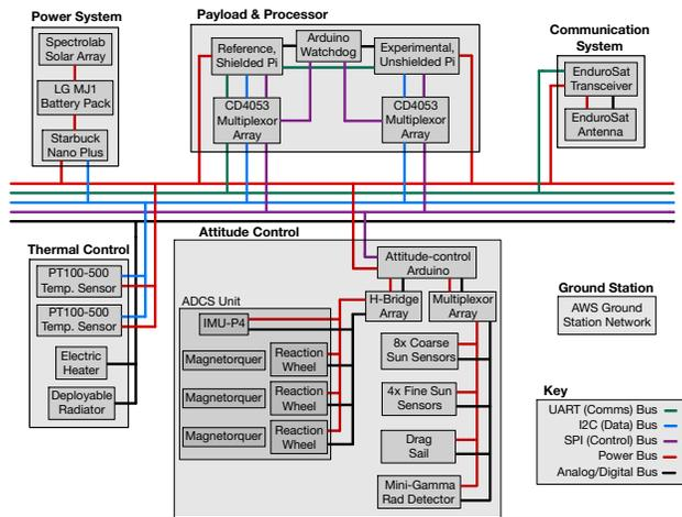
Figure 6. The functional block diagram, representing CLEOSATRA's design at the subsystem level.
