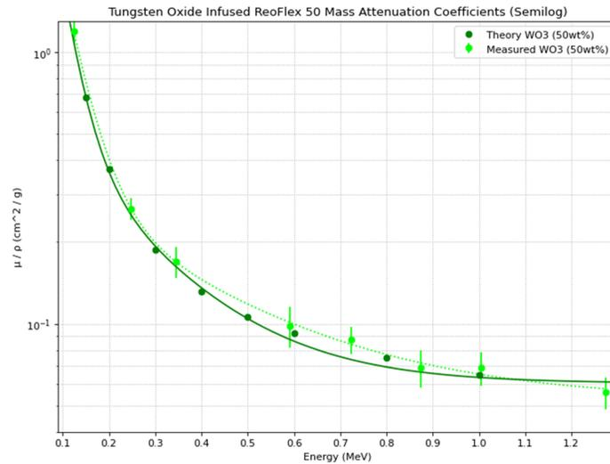
Figure 4. Tungsten oxide mass attenuation along typical energy levels.
