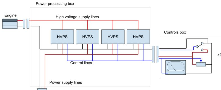
**Figure 9. High Voltage PPU (EN-4)**
