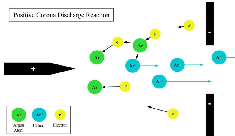
**Figure 3. Positive Corona Discharge Reaction**
