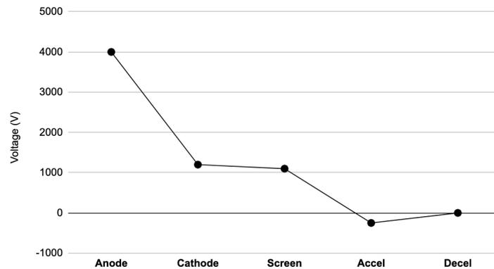
Figure 10. Voltage Bias of SG-2\_1 Prototype Components
