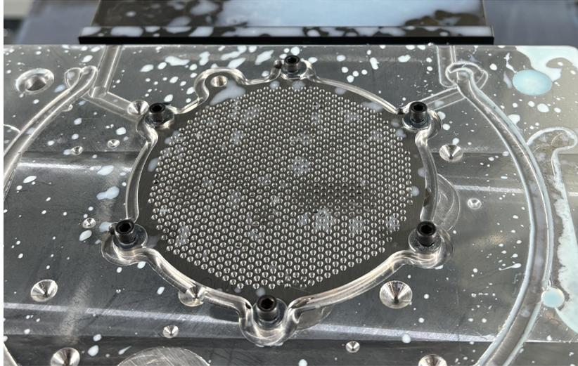
**Figure 11. Accelerator Grid Being Machined**
