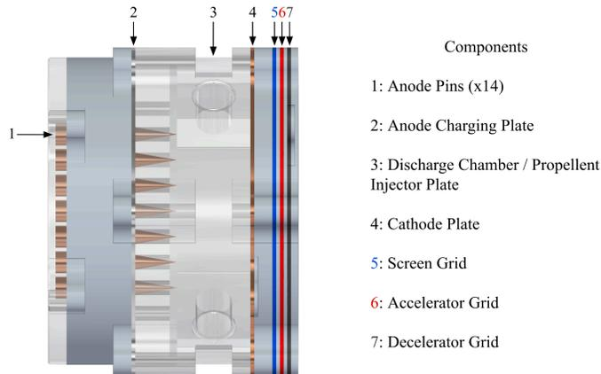
**Figure 6. SG-2\_1 Prototype Overview**
