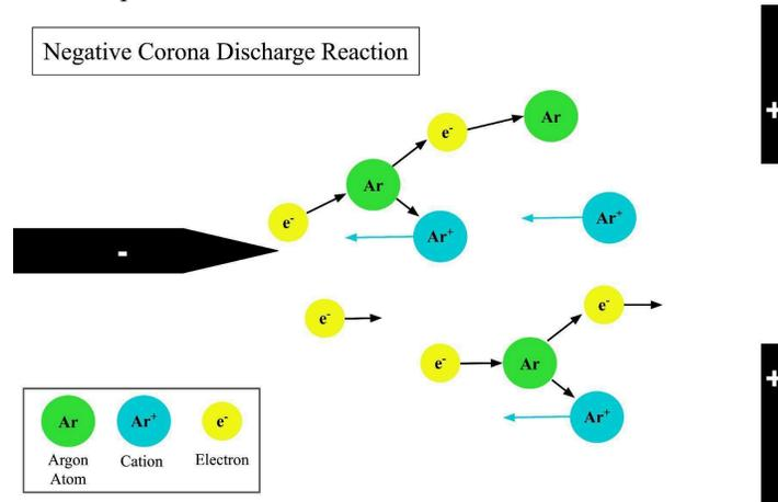
**Figure 2. Negative Corona Discharge Reaction**
