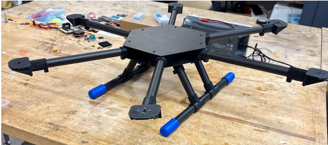
Fig. 5 Finalized Drone Design Excluding Electronics and Motors
