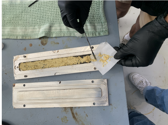
(a) Improved trial setup w/machine-cut fiber plies and evenly spread BDR
