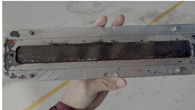
Figure 7. Composite compromised by CTE mismatch.
