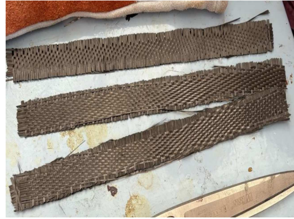
(b) Fully delaminated polymer matrix composite produced during first trial
