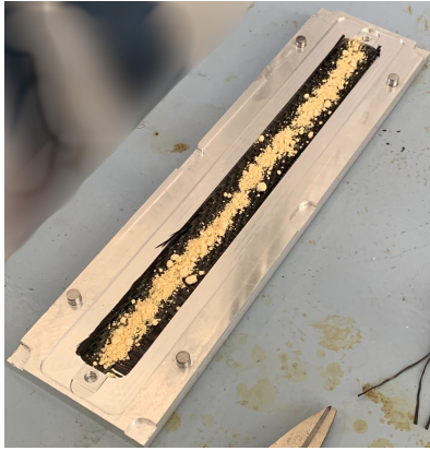
(a) First trial setup w/hand-cut fiber plies and under-spread BDR
