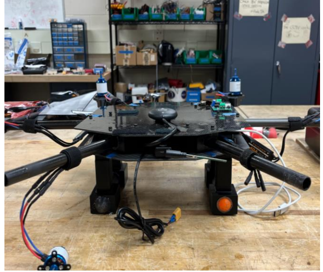
a) Fig. 2 a) Top view and b) rear view of the hexacopter showing the main plate, arms, and landing gear.
