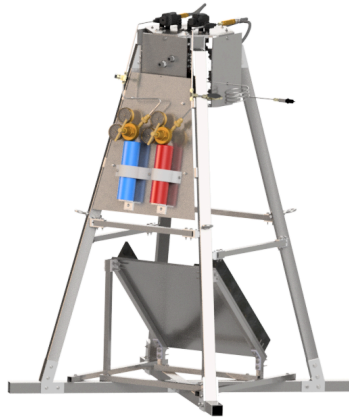
Fig. 1 CAD Model of the Engine Thrust Stand
