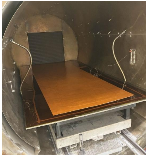
Fig. 12 AFP Panels Undergoing Consolidation via Autoclave
