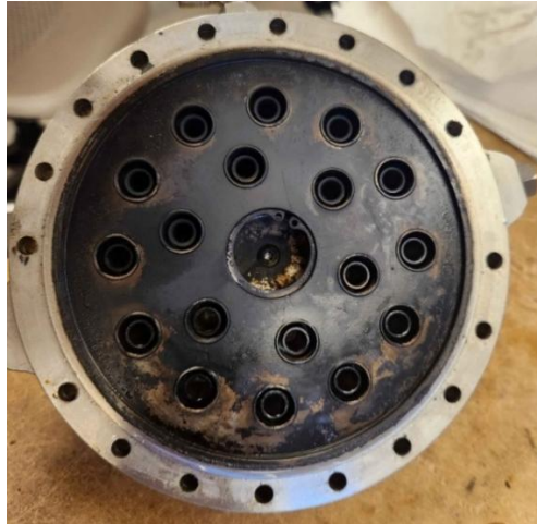
Fig. 18. Vespula injector faceplate post hotfire.
