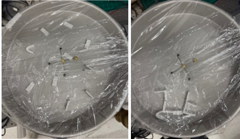
Figure 7. Before and After Shaker Test with S1016 Airfoil segments at 4V and 10 Hz
