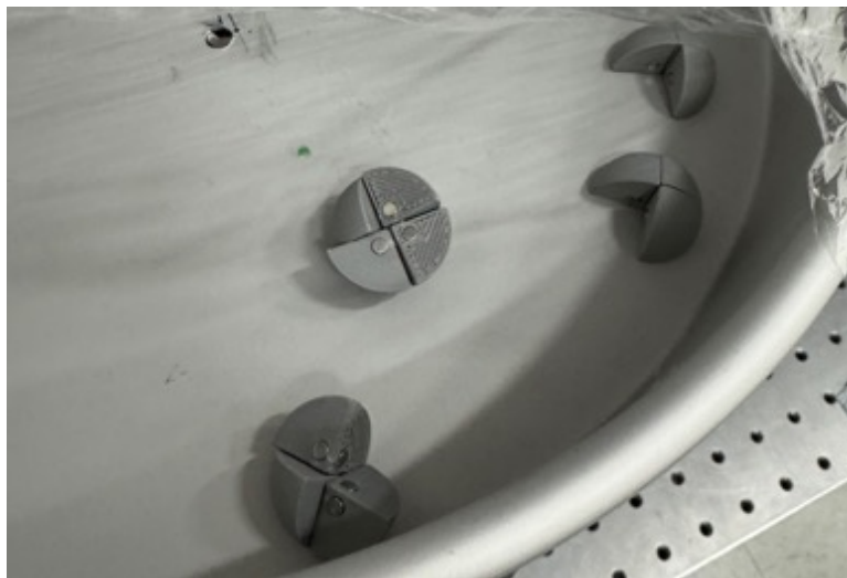
Fig 6. After of Shaker Test with Spherical Shapes at 4V and 15 Hz
