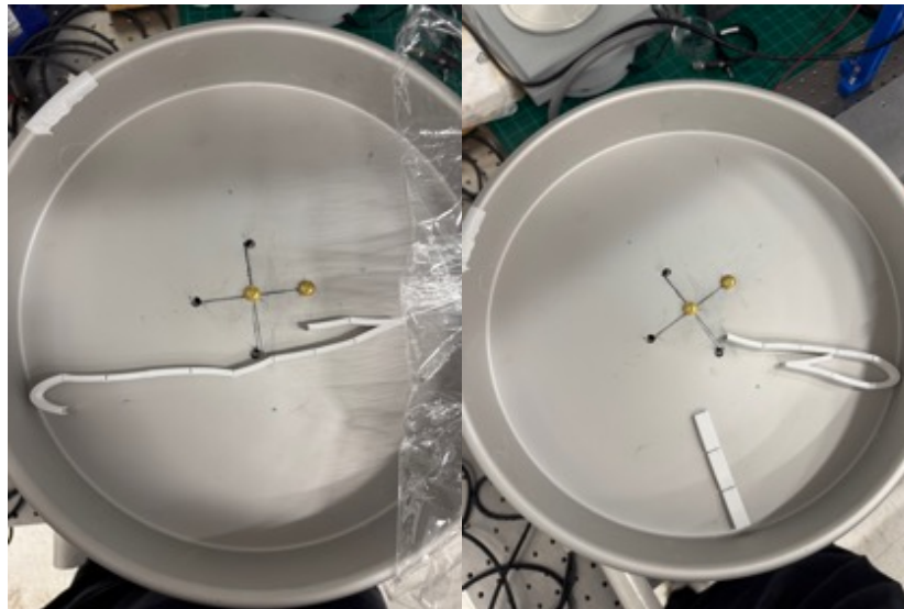
Figure 8. After of Shaker Test with S1016 Airfoil Segments at 6V and 10 Hz on the left and 6V and 15 Hz on the right
