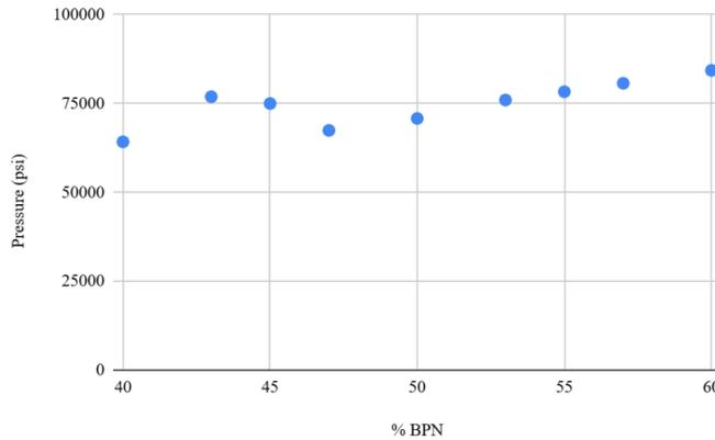
**Fig. 1 Percent Weight of BPN vs Pressure**
