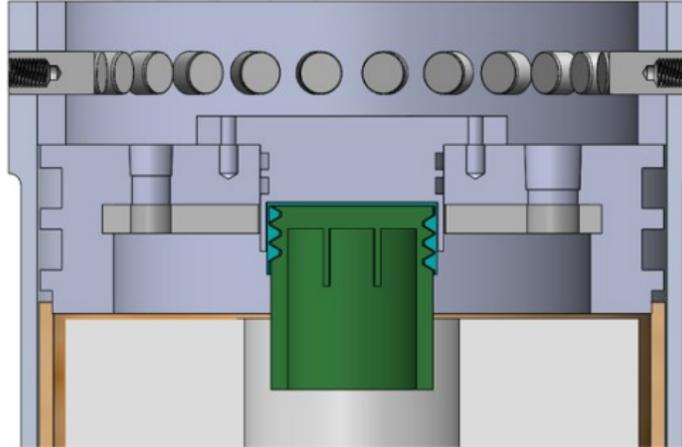
**Fig. 8 Forward Closure Integration with Igniter Puck**
