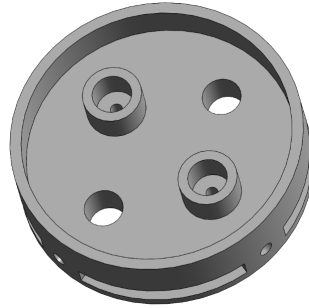
Fig. 9 Final recovery bulkhead (Top isometric view).
