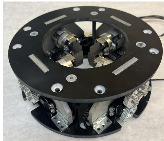
**Fig. 3 Fully assembled jet vanes assembly.**
