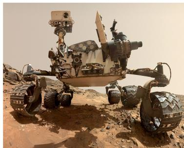
(b) NASA Curiosity rover used for planetary exploration and collecting samples on Mars.[6]
