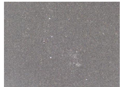
Figure 12. Optical view of coupon exposed to pumice at 5x magnification
