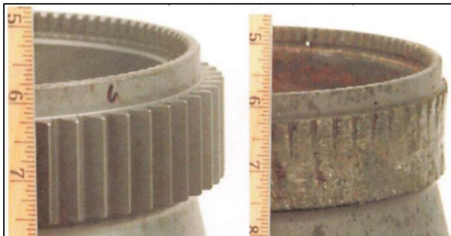
Fig 3. Gears Worn Down from CV-22 Osprey [7]
