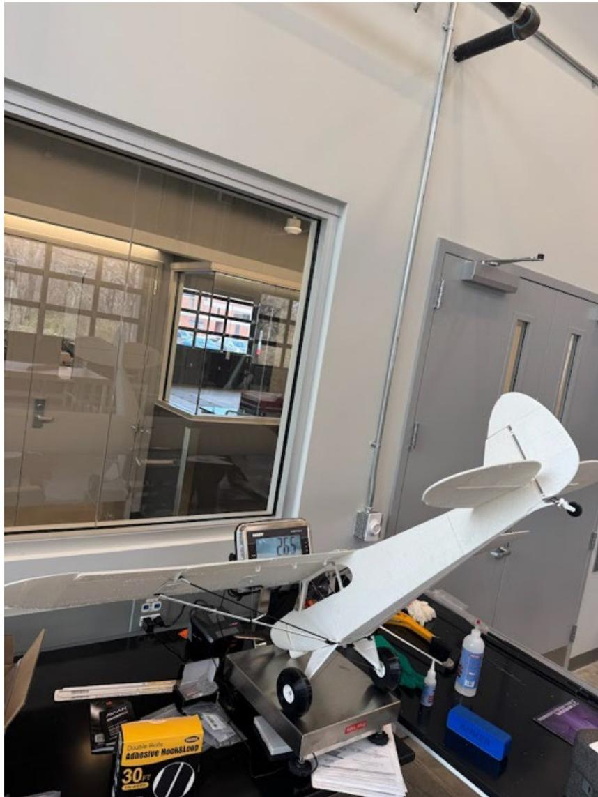
Fig. 3: Weight of Mothership (2.65 kg, Without Glider and Tanks)
