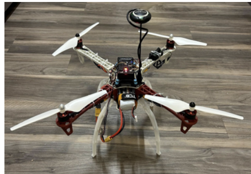
Fig. 2 Hawk's Work F450 Drone Assembled.
