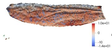
Fig. 3 Wing Bottom Pressure Distribution
