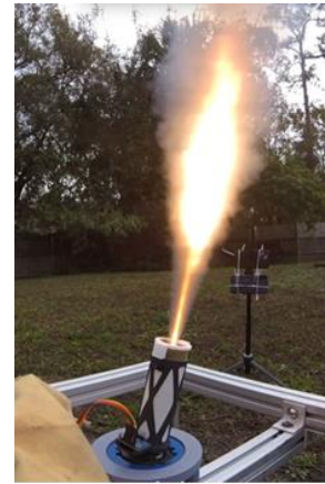
Fig. 21 TVC Mechanism Gimballed during Static Fire 2
