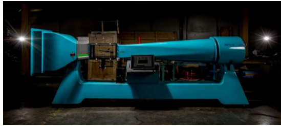
Fig. 16 AEROLAB Educational Wind Tunnel EWT used for data collection
