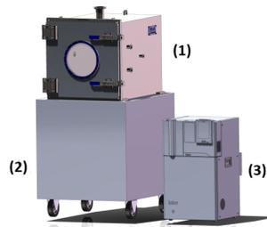
**Fig. 1 CAD model of the SEVC: Chamber (1), stand (2), and temperature control unit (3)[7, 8].**
