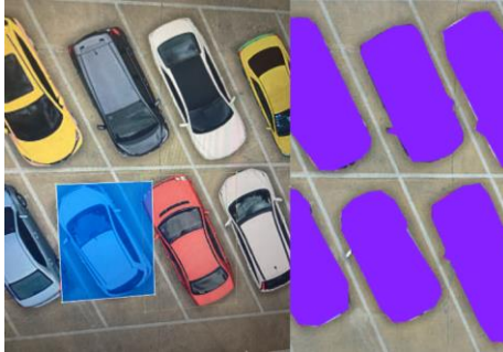
Figure 3: Object Detection bounding boxes vs. Image Segmentation masks for cars parked in angled spaces.
