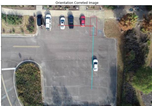
Figure 4: An image where PCA has been applied. The reference object in this case is the access aisle between the two handicap spots. Notice the major (x) axis (blue) is running lengthwise across the reference object while the minor (y) axis (red) runs parallel to the width.
