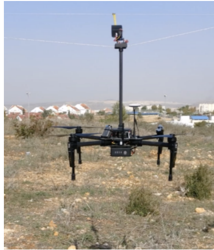
Fig. 3 Power line charging drone[6]
