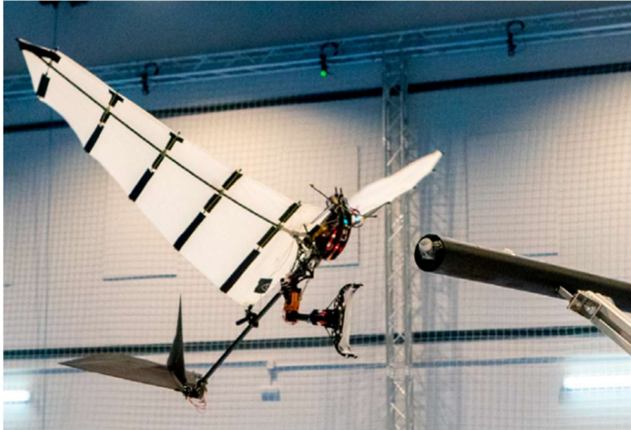
Fig. 4 Perching Mechanism on Ornithopters [2]
