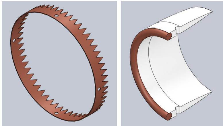
Fig. 2 Sawtooth Emitter Geometry (left) and the Section View of the Collector (right)
