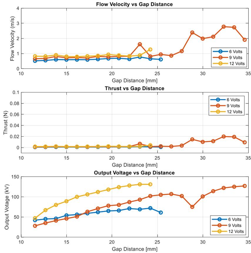
**Fig. 6 Graph showing Flow Velocity, Maximum Thrust, and Voltage Output vs Gap Distance respectively during Test 2**
