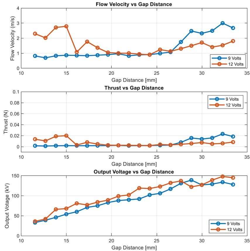
**Fig. 7 Graph showing Flow Velocity, Maximum Thrust, and Voltage Output vs Gap Distance respectively during Test 3**
