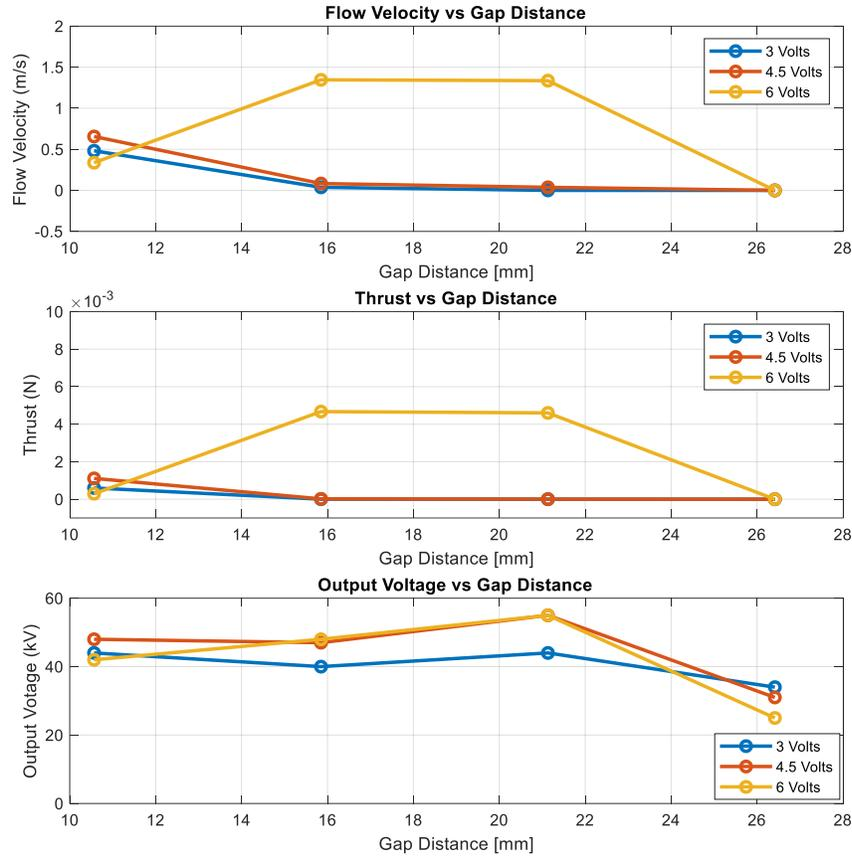
**Fig. 5 Graph showing Flow Velocity, Maximum Thrust, and Voltage Output vs Gap Distance respectively during Test 1**
