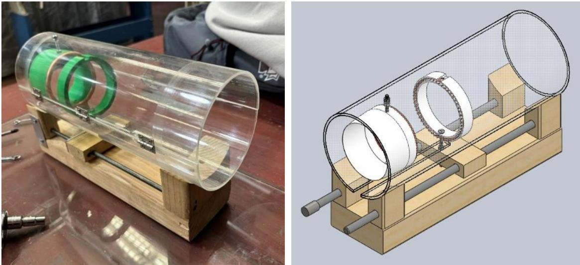
**Fig. 3 Testing Stand (left) and SolidWorks Model (right)**
