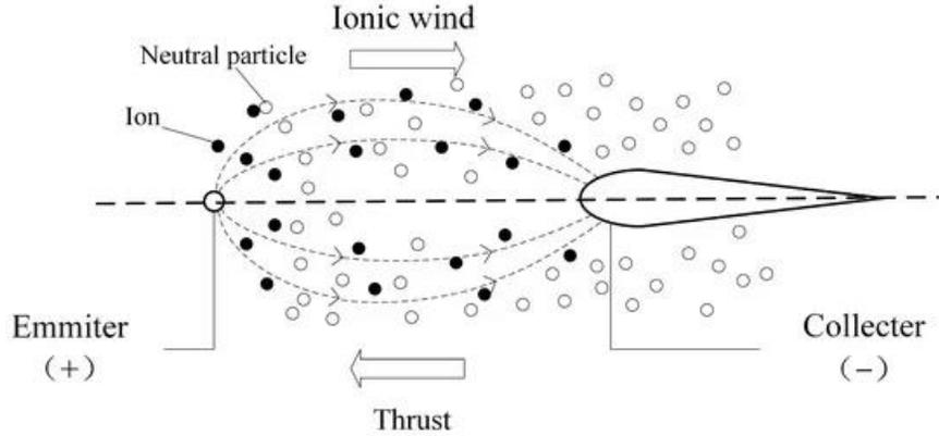
**Fig. 1 Ionization of Ambient Air and momentum Exchange [1]**
