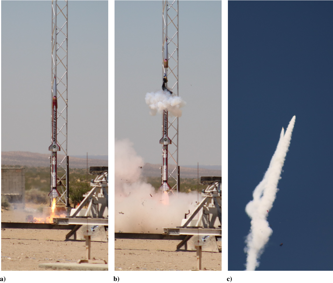
Fig. 7 Images of key flight events during liftoff of Material Girl : a) booster ignition b) premature nosecone deployment and c) sustainer hot staging. Courtesy of Casey Wilson.
