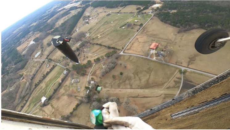
Fig. 5 Drop test article being released from Cessna 208 aircraft at 460 m AGL during first drop test
