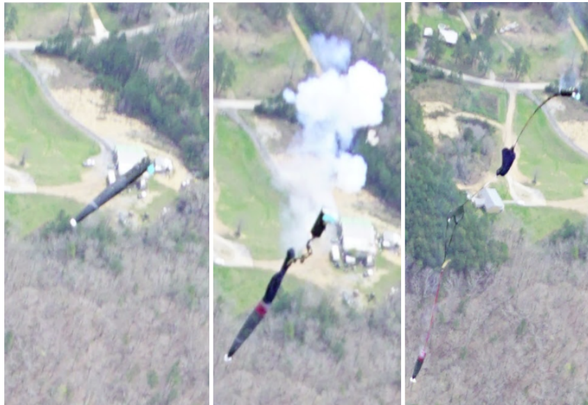
Fig. 9 Sequence showing test article deployment. The first image shows the test article under freefall pre-separation. The second image shows the article moments after separation, with the airframe parachute protector visible. The last image shows the nose cone parachute and parachute protector.
