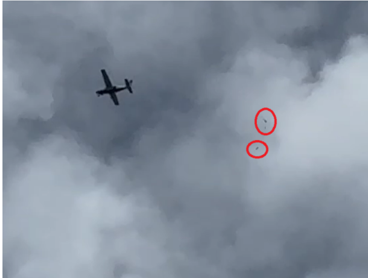
Fig. 8 Nosecone (lower) and airframe (upper) falling away from airplane after deployment during the second drop test.
