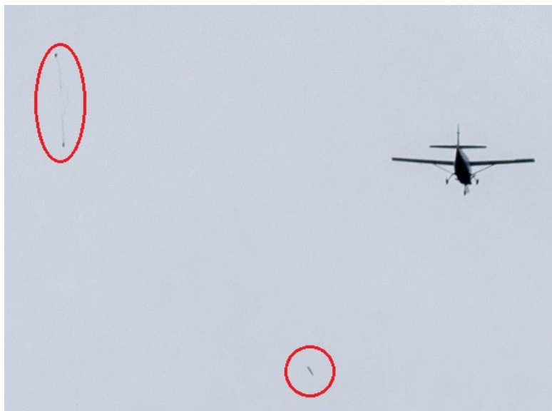
Fig. 6 The drop test airframe (top left) and nosecone (bottom) falling away from the airplane during the first drop test.
