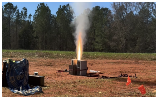
Fig. 4 GT-ARES Propellant Hot Fire Test.
