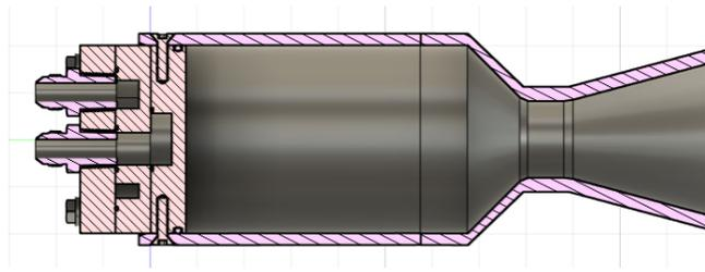
**Fig. 6 CAD Design of Chamber and Nozzle.**
