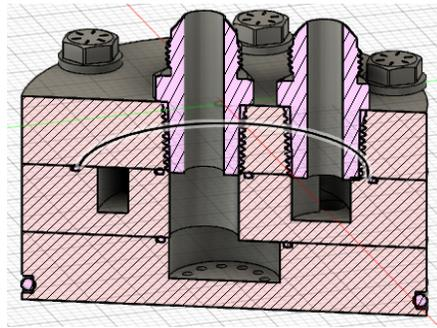
**Fig. 3 CAD model of final injector design, section view.**
