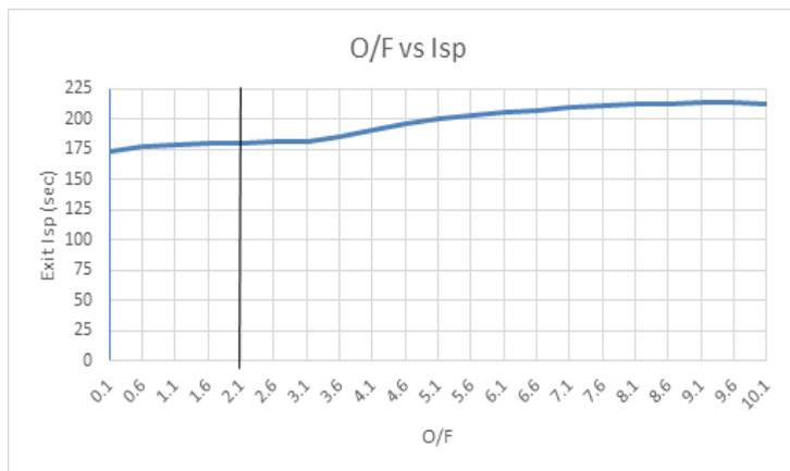
**Fig. 4 Oxidizer/Fuel ratio vs exit  $I_{sp}$  (sec).**
