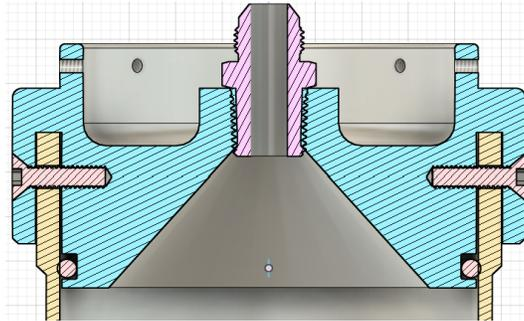
**Fig. 7 Cross-section of final assembly of bulkhead and tank.**
