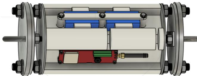
**Fig. 8 Complete avionics bay design.**
