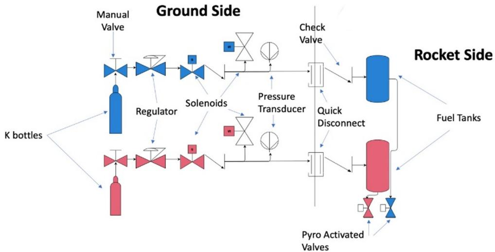
**Fig. 11 Ground Systems Architecture**
