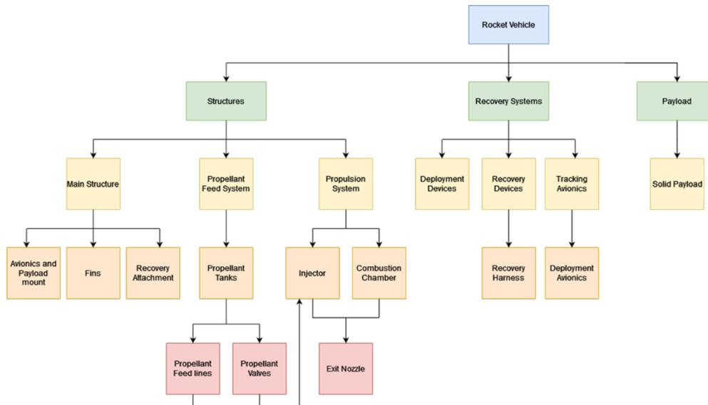
Fig. 2 BiProp systems architecture flow chart.
