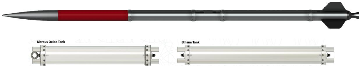
**Fig. 1** Full rocket with nitrous oxide tank (*bottom left*) and ethane tank (*bottom right*)
