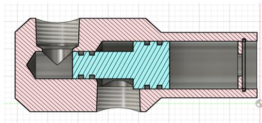
**Fig. 10 Valve Assembly Cross Section.**
