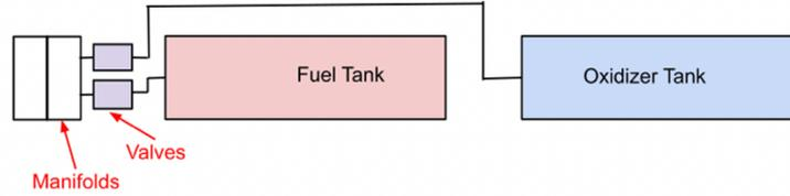
**Fig. 9 Basic Fluid System Layout.**
