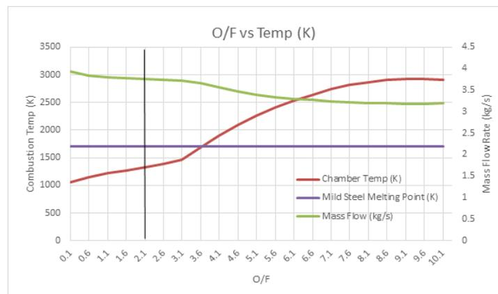
**Fig. 5 Oxidizer/Fuel ratio vs. combustion temperature (K).**
