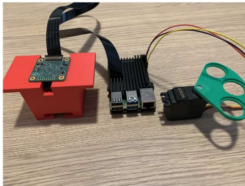
Fig. 4 Raspberry Pi camera [5] connected to Raspberry Pi 4 [9] via ribbon cable with TowerPro servo [8] connected via IO pin 18. Camera is held in place by ground test model, and servo supports filter holder.
