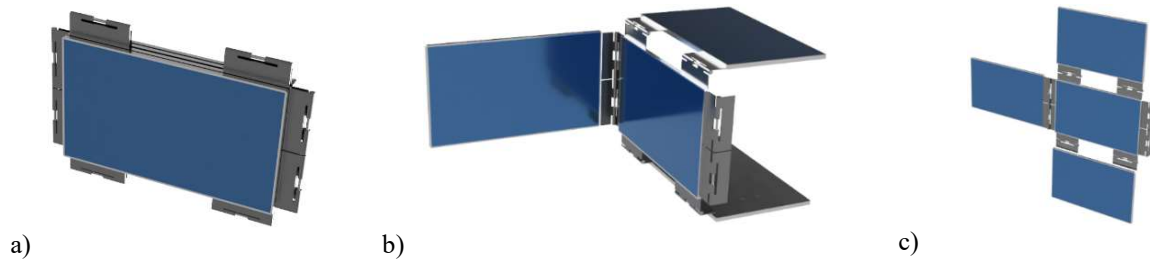
Fig 7: Folded (a), deploying (b), and deployed (c) 4x solar array.
