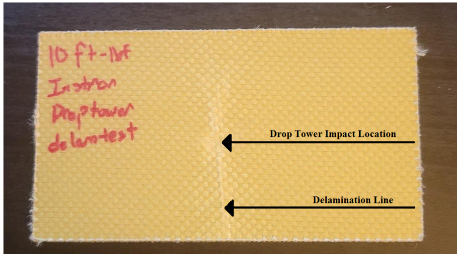
Fig. 3 Unstitched Kevlar ® coupon after drop tower impact at 10 ft-lbf
