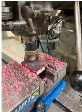
Fig. 10 Cast samples being faced on Bridgeport knee mill.
