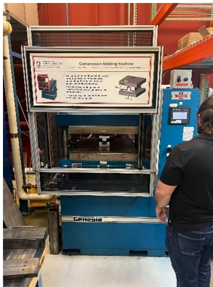
Fig. 8 Wabash hot press being set up to run the aluminum tool.
