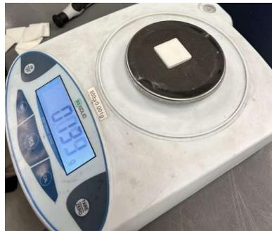
**Fig. 10 Sand Weighing Method using Scale**
